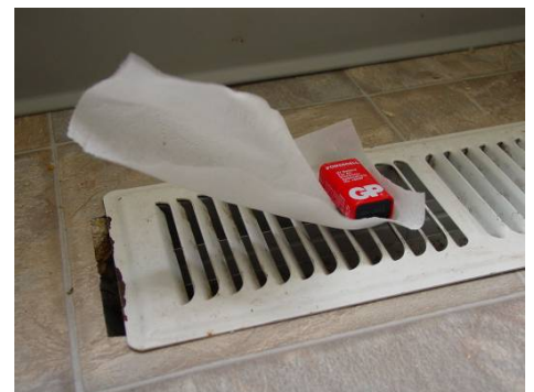
Figure 1141-3: Sometimes duct leakage is obvious before you use the pressure pan; air coming out of a register with blower door operating; air handler is not on!
