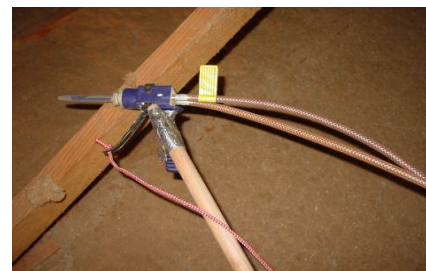
Figure 2122-12: 2-part spray foam gun secured to broom stick with string attached to handle
