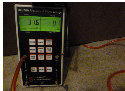
Figure 1152-1: Room to room pressure is 31.6 Pa!
