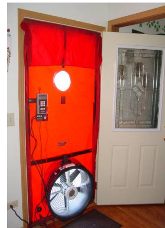
Figure 1112-1: Blower door set-up
