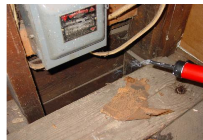
Figure 2121-1: Smoke being drawn down an open study cavity indicating leakage to the inside
