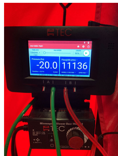
Figure 11121-1: CFM50 is displayed when 50Pa cannot be achieved in a home
