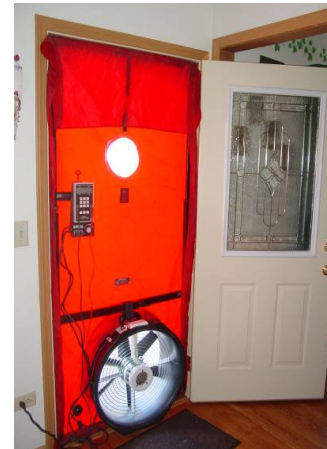
Figure 1112-1: Blower door set-up
