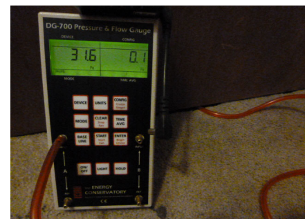
Figure 1152-1: Room to room pressure is 31.6 Pa!
