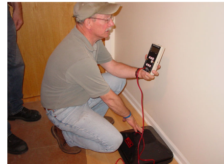
Figure 114-1: Pressure pan test
