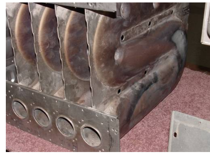
Figure 3151-1: Furnace heat exchanger
