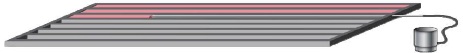
Figure 4142-2: Insulating floor cavity from the end where the floor joists run the length of the mobile home (end blow)
